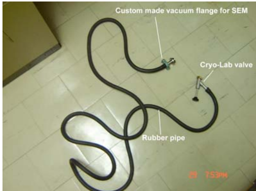
Figure 1: Cryo-Lab valve, custom made vacuum flange for SEM and rubber pipe.
