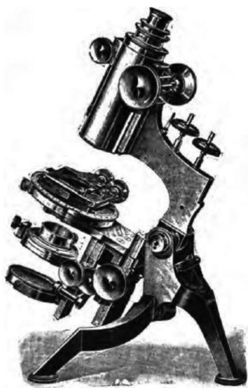
Fig. 86. — Metallurgical microscope constructed by Watson and Sons.
