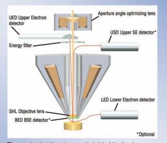
The newly developed super hybrid objective lens (SHL) provides the resolution of 0.8nm at 15kV and 1.2nm at 1kV. The SHL objective lens allows researchers to study various samples at high magnification.
