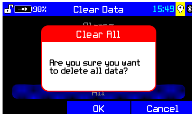
Figure 6-75: The system prompts the user for confirmation; press R (Cancel) to return to the Clear Data menu
