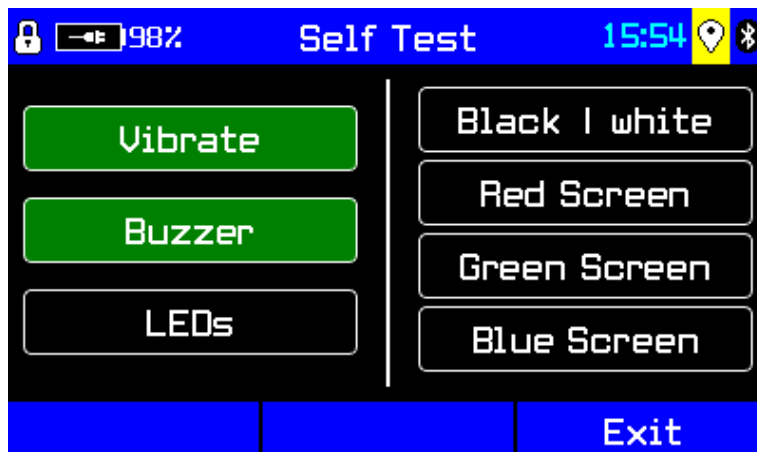
Figure 6-48: Testing all notifications: The system has cycled through Vibrate and is verifying the buzzer
