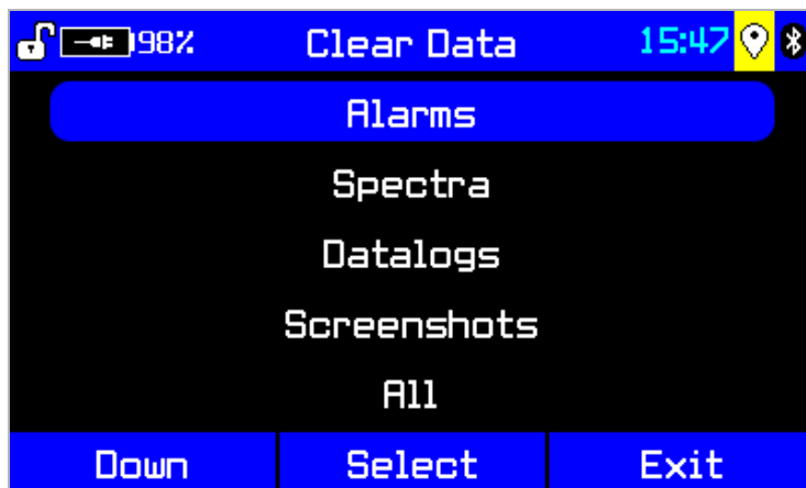
Figure 6-70: From the Clear Data menu, select Alarms to clear all saved alarms
