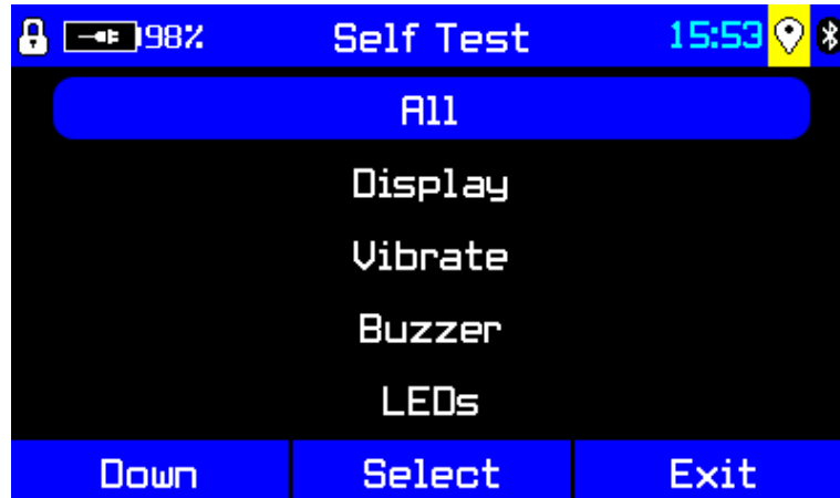
Figure 6-46: Select All to test all functions listed below, or select an option to test individually
