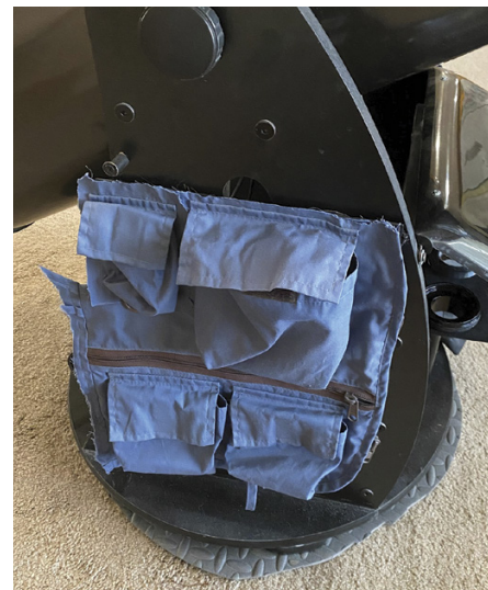
▲ A section of a fishing vest is attached to the adjacent side of the Dobsonian's rocker box with Velcro. It serves as a handy collection of pockets for onboard storage of assorted observing gear such as eyepieces, headlamp, spare batteries, red flashlight filters, etc.
