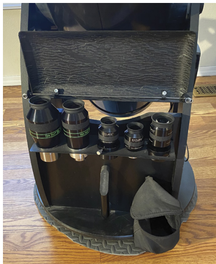
▲ Lauren's modified eyepiece rack features a flip-down lid to shield the eyepieces from dew. Also seen is a rubber mat to protect the scope's particleboard base from the damp ground and a small bag to safely stow knobs and fittings so they don't get lost in the dark.
