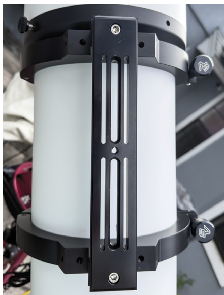
▲ A plate connecting the top of the machined tube rings is slotted to facilitate connecting additional accessories, including tube rings for a guide scope or other ride-along devices like a minicomputer.
