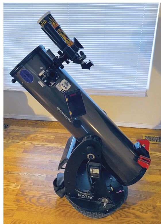
▲ Lauren Wingert's heavily modified Orion XT10i Intelliscope reflector. About a third of her modifications are visible here, including the two oversized finderscopes and the red welding magnetic holders as extra counterweights.
