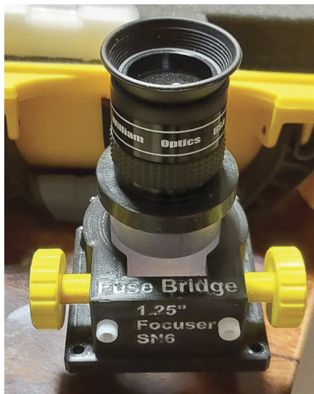
▲ Telescope maker Sasha Demenko 3D-printed and assembled this Crayford-style focuser, which required some bushings, bearings, and a polycarbonate tube.
