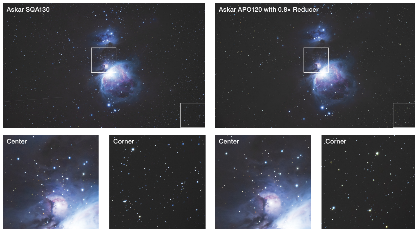
▲ These single frames — shot on consecutive nights at the same times and with the same camera — attempt to show the difference in star sharpness between the Askar SQA130 and the Askar APO120 with its 0.8× reducer. It takes pixel-peeping to see a difference, mostly in the corners.
