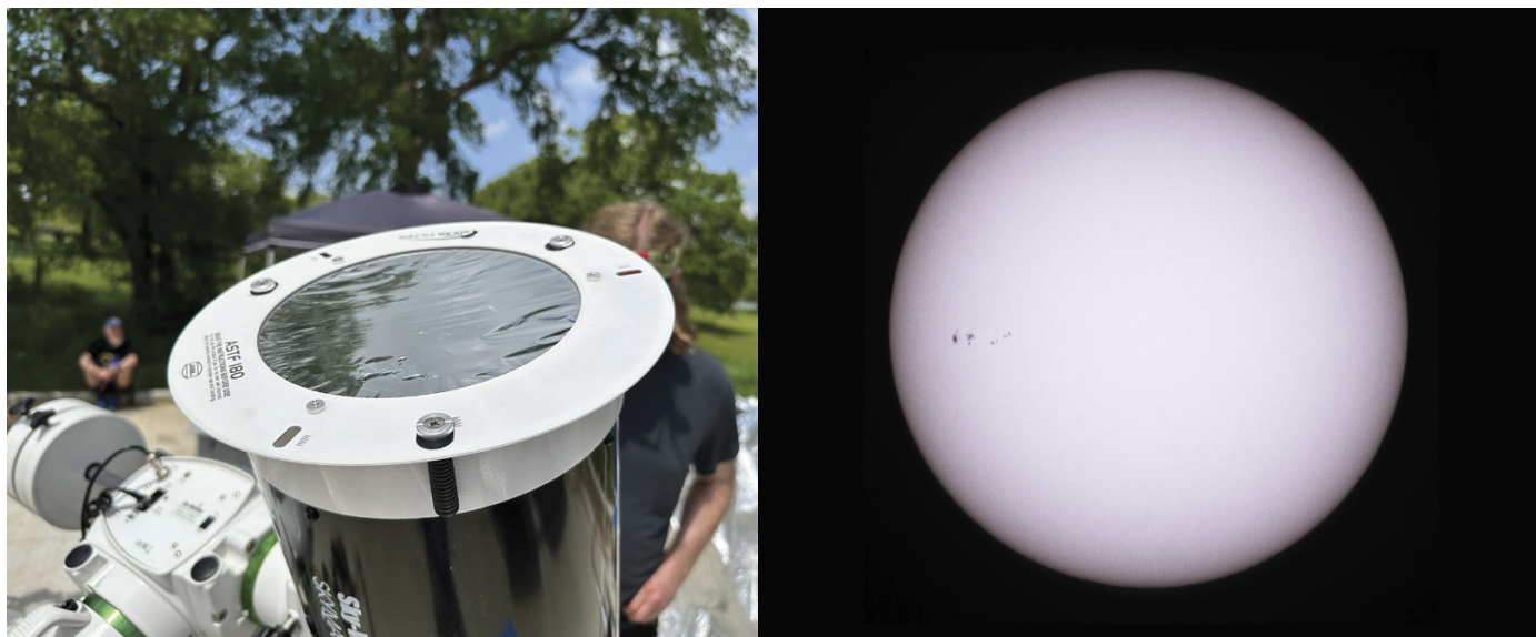
▲ WHITE-LIGHT GATEWAY Front-mounted solar filters, like this example from Baader Planetarium (left) using optical-quality polymer film, are the most affordable entry into solar observing by making a telescope you already own safe for solar viewing. These filters are sold in sizes for telescopes of up to 280 mm and produce a view of the photosphere revealing sunspots, plages, and granulation (right).
