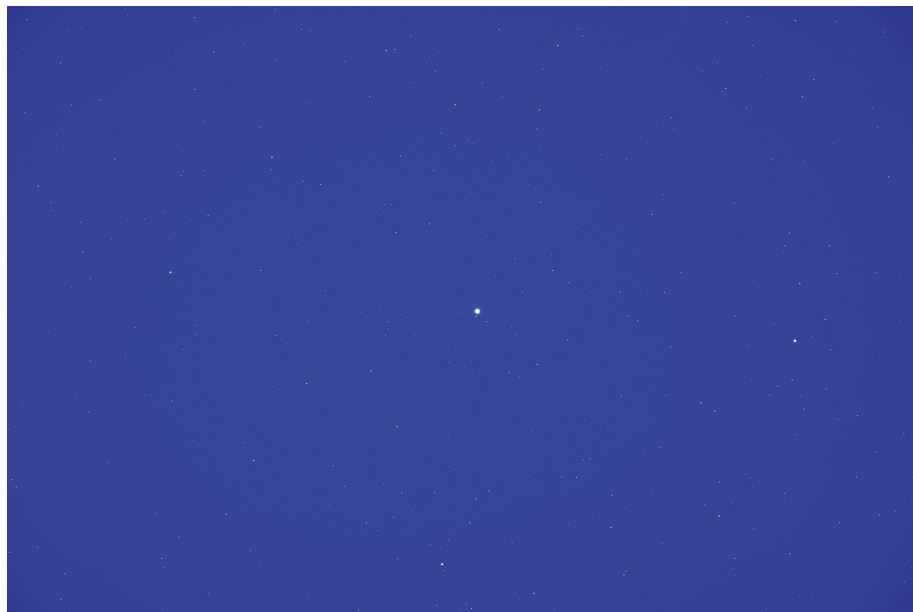
▲ A single exposure of Castor, Alpha ( \alpha ) Geminorum, in twilight and with the contrast boosted shows a fairly uniform field illumination, except for a slight darkening at the extreme corners.
