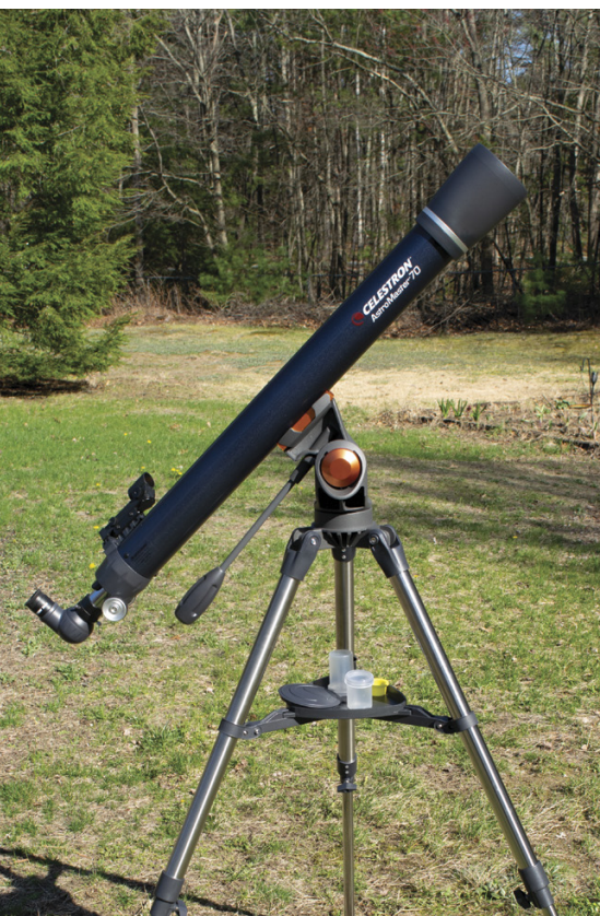
▲ The Celestron AstroMaster 70AZ is a long-focus achromat with a sturdy, easy-to-aim alt-azimuth mount.
