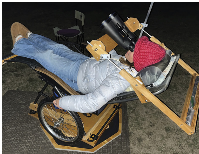
▲ Left: Reclining the chair raises the binoculars toward the zenith while preserving eye alignment, making overhead observing unusually easy and comfortable. The user moves in azimuth by turning the steering wheel mounted on the side of the chair. Right: Dave demonstrates the bino-chair at the 2023 Stellafane Convention in Vermont. (To see another design variation, using a car bucket seat, see the August 2024 issue, page 74.)
