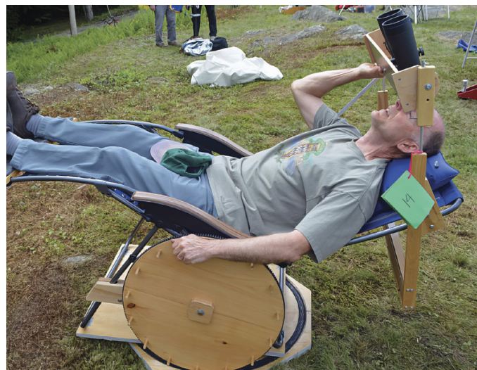
▲ Left: Reclining the chair raises the binoculars toward the zenith while preserving eye alignment, making overhead observing unusually easy and comfortable. The user moves in azimuth by turning the steering wheel mounted on the side of the chair. Right: Dave demonstrates the bino-chair at the 2023 Stellafane Convention in Vermont. (To see another design variation, using a car bucket seat, see the August 2024 issue, page 74.)
