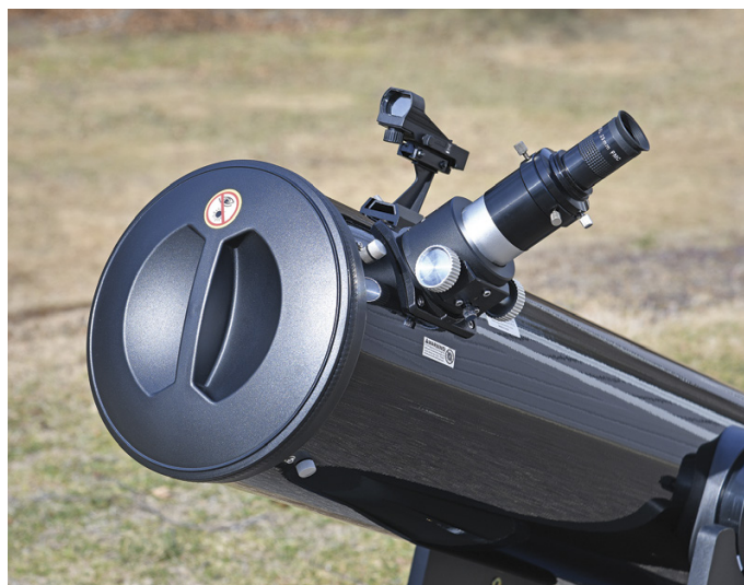
▲ Left: A tight-fitting plastic cover protects the telescope optics from dust and pollen during transport and storage. Right: The scope's primary-mirror cell has a rim that extends farther out than the mirror's collimation knobs and locking thumbscrews, allowing the tube to be placed upright on the ground without fear of disturbing the collimation. The rim also served as a convenient place for the author's small, clip-on counterweights that he needed for balancing the scope when using heavy eyepieces.
