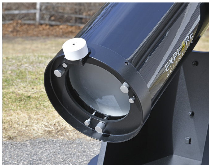
▲ Left: A tight-fitting plastic cover protects the telescope optics from dust and pollen during transport and storage. Right: The scope's primary-mirror cell has a rim that extends farther out than the mirror's collimation knobs and locking thumbscrews, allowing the tube to be placed upright on the ground without fear of disturbing the collimation. The rim also served as a convenient place for the author's small, clip-on counterweights that he needed for balancing the scope when using heavy eyepieces.
