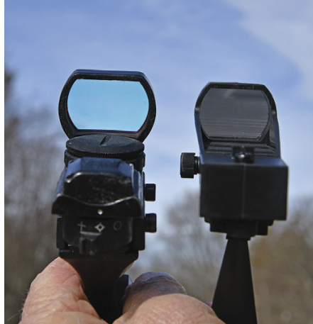
▲ A dark coating on the "window" of the scope's supplied red-dot finder (right) is seen here next to a far-more transparent finder from a 20-year-old Meade Lightbridge telescope. [Editor's note: After this review was completed, Explore Scientific announced that a different red-dot finder will be supplied with this scope in the future.]
