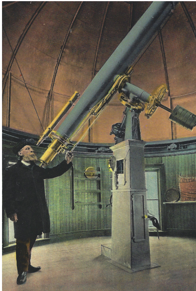
▲ COMET HUNTER William R. Brooks stands with his 10 \frac{1}{8} -inch refractor. John Clacey built the optical assembly; the equatorial mount and dome are by Warner & Swasey. Mounted in 1888, it is still the main telescope of the Smith Observatory in Geneva, New York.
