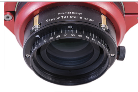
▲ The rear cell includes a plate for adjusting the tilt of the camera, using four wheels (two are visible here) at 90° spacing, which are turned with a 2-mm Allen wrench.
