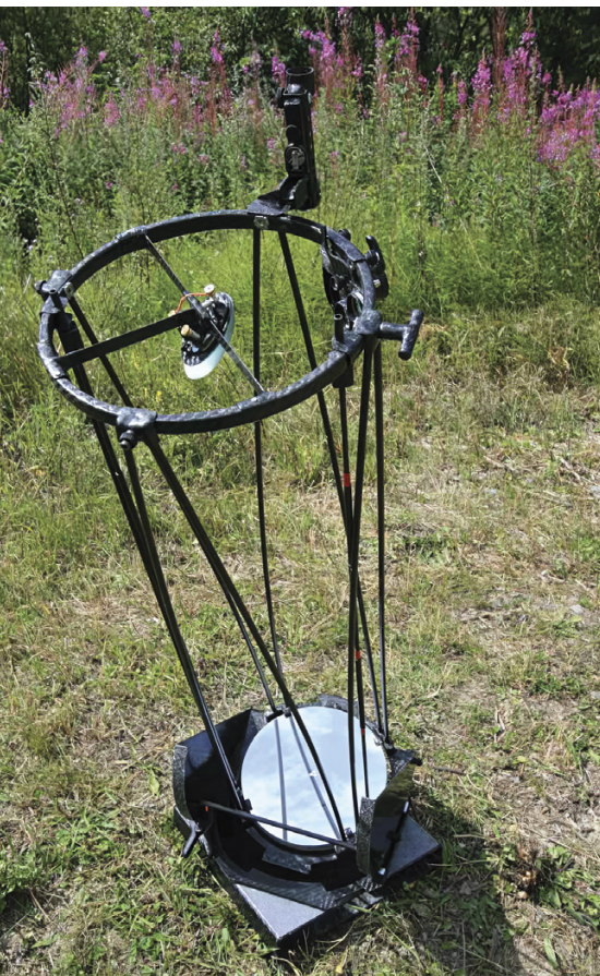
◀ Laurent Bourasseau's innovative 250-mm (10-inch) f/4.5 truss Dobsonian is fully assembled and ready for observing.
