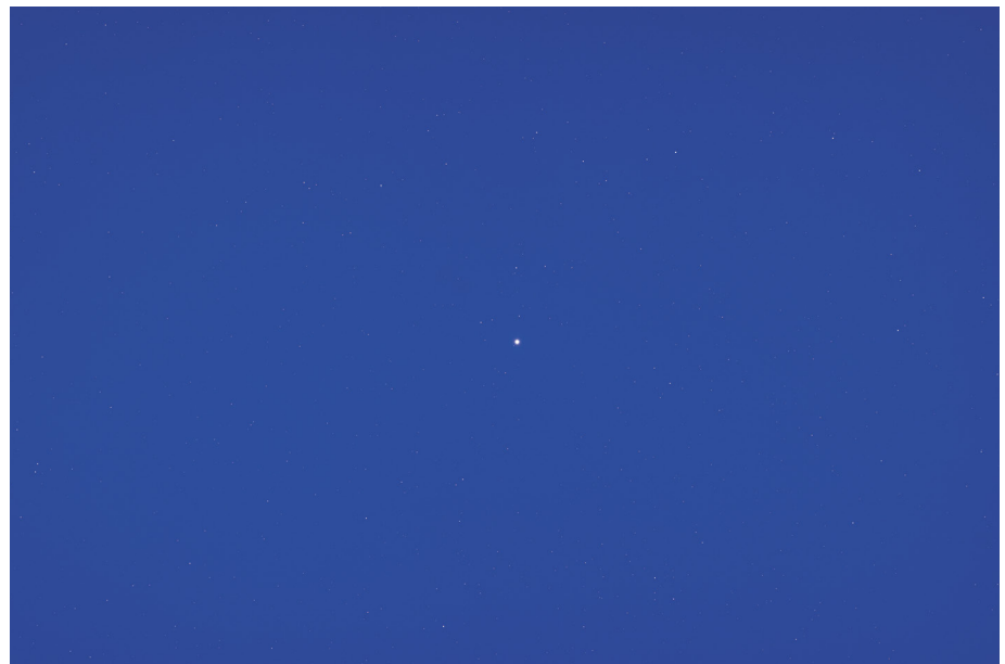
▲ Taken in deep twilight and with the contrast boosted considerably in processing, this image of the region surrounding +0.1-magnitude Capella (Alpha Aurigae) shows the scope’s fairly uniform field illumination, with only minor and gradual darkening toward the corners of a full-frame sensor.
