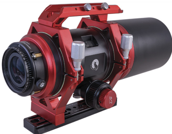
▼ Left : The mid-tube internal focuser shifts the optics within the tube more than 21 mm. A window on the tube shows its position, here at 0 mm, with the rear lens closest to the end of the scope. Right : The mid-tube focuser has a lock and bolt holes to accept an electric focus motor. The Vixen-style dovetail bar can be shifted over a range of 70 mm to aid balancing the telescope.
