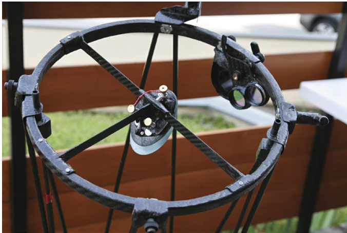
▲ Left: The upper cage assembly is shown with the secondary mirror attached via magnets. Laurent notes that the detachable secondary saved lots of space when packed. The spider, filter slide, focuser board, finder, and truss fittings all pop off for travel as well. Right: The Slim250 is seen partially dismantled for transport. From bottom to top, we see the rocker base with Teflon altitude pads; the large ring just inside this is the upper cage, surrounding the lower cage with truss blocks visible. The primary mirror here is safely ensconced in a carbon-fiber lid. The altitude bearings, monolithic composite hulls with laminate rims, nest snugly over this.
