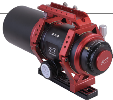
▲ The tube rings include six M6-threaded holes for adding a top accessory plate. They include riser blocks providing 50 mm of spacing between the scope and dovetail plate.
