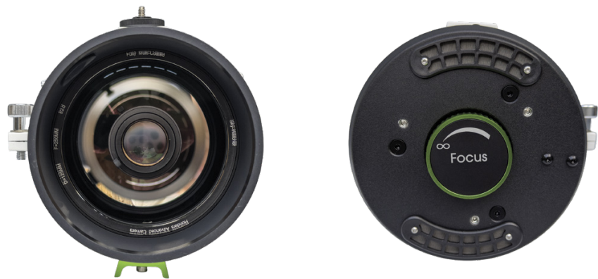
▲ Left: Looking down the tube reveals the primary mirror as well as the final corrector where the camera is mounted. A thumbscrew at lower left secures the camera when connected to one of the three included adapters. Right: The rear of the Minigraph features a large focusing knob surrounded by two trios of collimation screws; the black ones move the primary mirror while the silver screws lock the mirror's position. Two vents in the upper and lower sections help the optics reach ambient temperature quickly. The pair of black screws at right are used to mount third-party focus motors.
