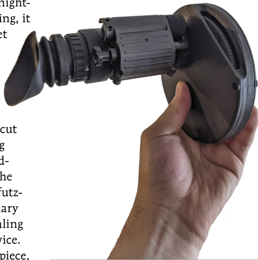
▲ The author's 3D-printed, fully assembled apparatus is shown here with the PVS-14 Gen 3 Night Vision Monocular mounted securely to the filter wheel adapter system.
