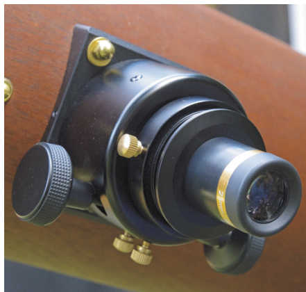
▲ Left: The darning hoop tube ring and finderscope are styled to match — a brass chain secures the lens caps (one of which was pulled from a Karo syrup bottle). Right: Snow replaced the hardware on her commercial focuser with brass thumbscrews, which sells the whole nautical effect swimmingly.
