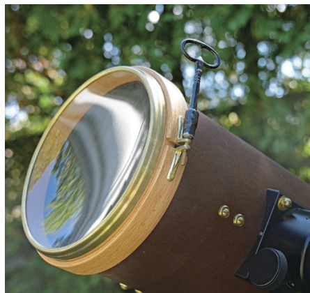
▲ Left: A darning hoop and a serendipitously snug bezel from a banjo clock together make up the dust cover. Middle: An antique doorknob caps the counterweight shaft. Right: Parts from an antique chair, a window, and other scavenged bits form the altitude and azimuth adjustments for this scope. The counterweight shaft juts out at an odd angle, allowing the scope to reach low-altitude targets.
