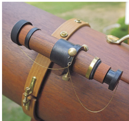
▲ Left: The darning hoop tube ring and finderscope are styled to match — a brass chain secures the lens caps (one of which was pulled from a Karo syrup bottle). Right: Snow replaced the hardware on her commercial focuser with brass thumbscrews, which sells the whole nautical effect swimmingly.
