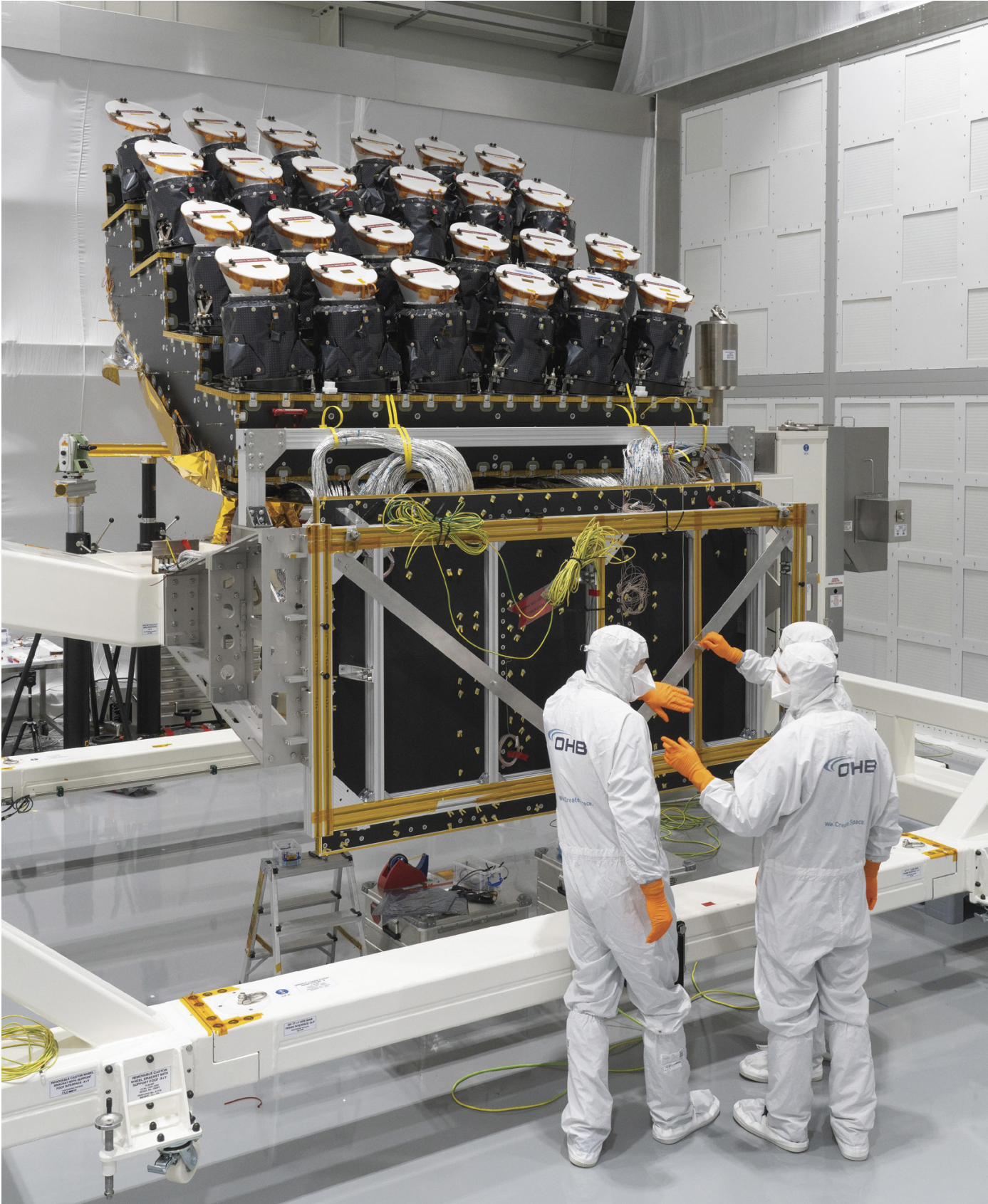
▲ UNDER CONSTRUCTION Engineers inspect PLATO's 24 newly installed cameras on the spacecraft's optical bench, which keeps all the cameras firmly pointed in the right direction. (The two “fast cameras” were still to be installed when this photo was taken.)
