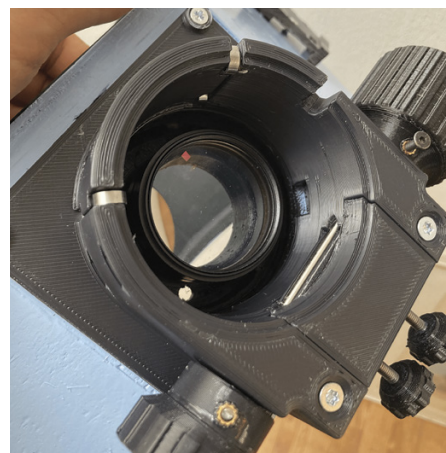
▲ Left: The upper tube assembly of Kermit II showing Lucas’s homemade 2-inch filter slide and dual-speed Crayford focuser. Middle: This cutaway view shows the guts of the focuser. Note the threaded adjuster that the coma corrector screws into and the homemade filter slide. Right: The focuser seen with its drawtube removed to show the embedded coma corrector mounted at a fixed distance. This arrangement makes each eyepiece come to focus at the proper spacing for the corrector to be most effective.
