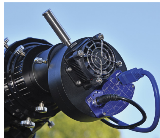
► The rear of the camera housing contains the power port and USB 3.0 connection. Also visible is the fan mounted on the heatsink fins for the camera's thermoelectric cooler.
