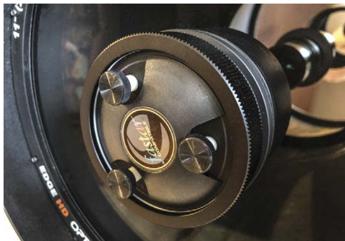
▲ TOOL-FREE COLLIMATION Replacing the stock collimation screws with ones from Bob's Knobs enables tool-free collimation adjustment of a Schmidt-Cassegrain secondary.
