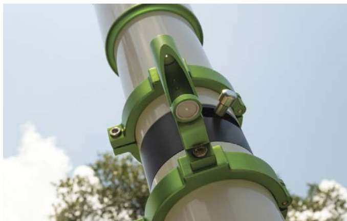
▲ A clever solar finder comes attached to the carry handle that bridges the tops of the tube rings. It works by projecting a small image of the Sun onto a frosted screen. The disk is visible from the focuser end of the scope ( right ) or when standing aside the objective lens ( left ).
