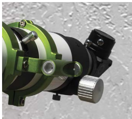
▼ Left: Tuning the etalon is achieved with the silver Trifid Tuner lever in the middle of the tube between the two tube rings. Middle: The 1 1/4-inch-format, 90° diagonal contains an 11.5-mm blocking filter, which is an integral part of the filtering system. Right: The scope includes a 2-inch, dual-speed Crayford-style focuser with 1 1/4-inch eyepiece adapter that firmly holds focus with a variety of eyepieces and cameras.
