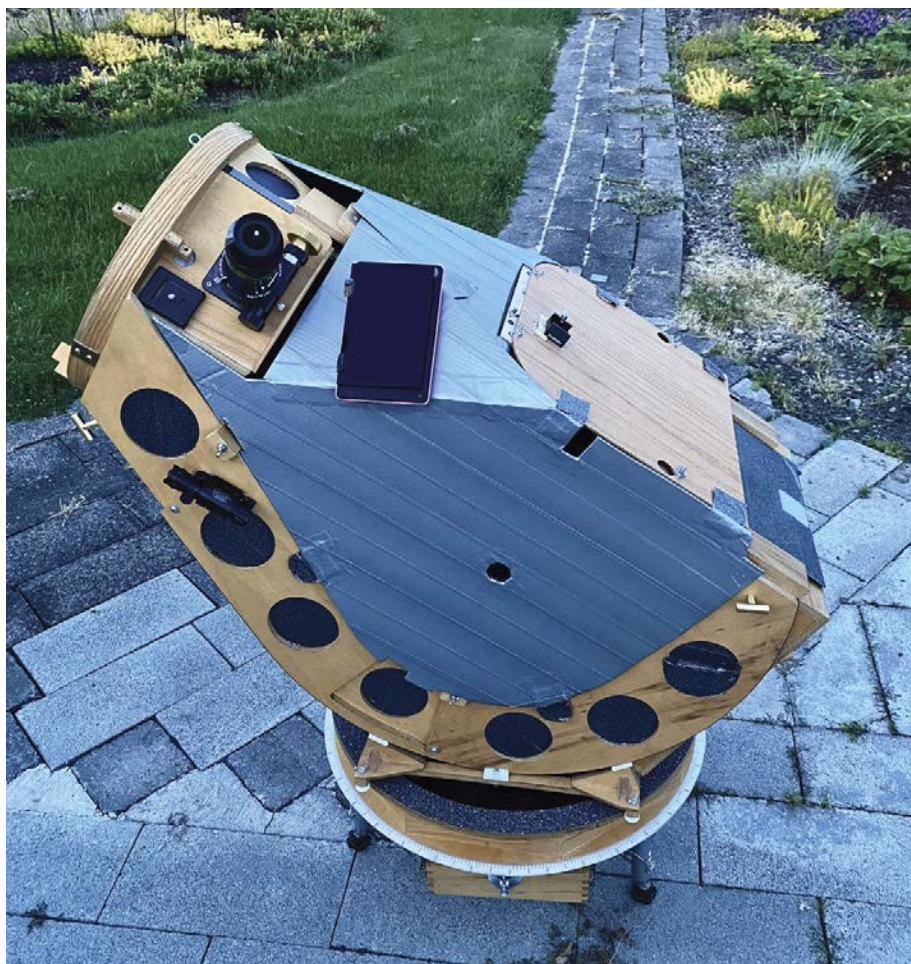
▲ Lauren’s solution for the Zip Dob is a custom-fitted, corrugated-plastic panel with flocking on the interior faces.
