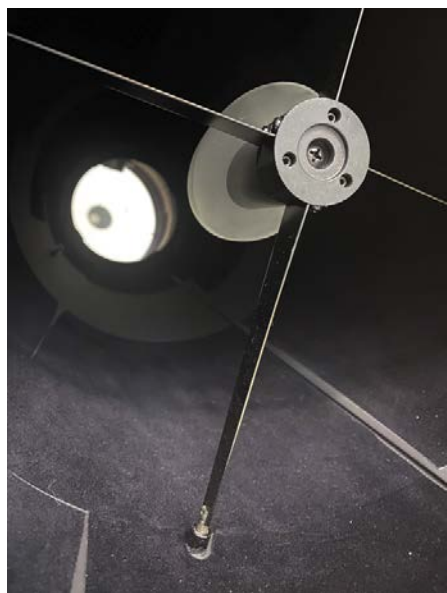
▲ The dark interior of Lauren's XT10i Intelliscope — note that the gaps in the flocking show how much darker her finish is compared to the original paint.
