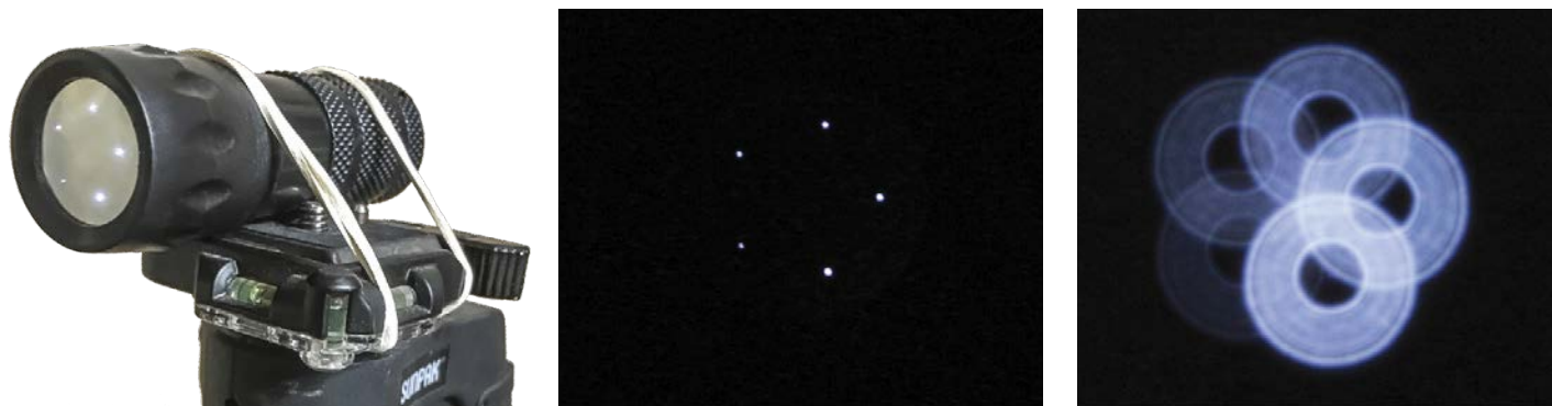
▲ STARS ON DEMAND The Hubble Optics 5-Star Artificial Star is as small as a pocket flashlight and is easily affixed to a tripod with a rubber band for positioning in front of the telescope at the appropriate distance ( left ). It produces five points of light with increasing brightness levels ( seen at center and right ). Unused stars are then covered with an included magnet (not shown).
