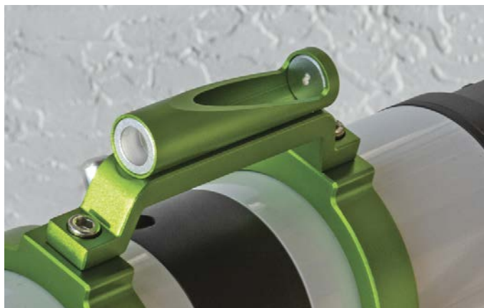
▲ A clever solar finder comes attached to the carry handle that bridges the tops of the tube rings. It works by projecting a small image of the Sun onto a frosted screen. The disk is visible from the focuser end of the scope ( right ) or when standing aside the objective lens ( left ).
