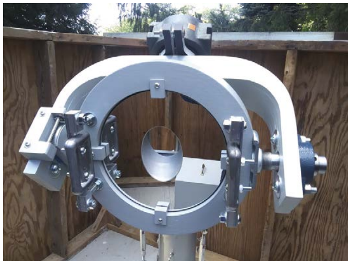
▲ Left: On the left side of the fork, a lag screw interfaces with a modified hose clamp to provide declination axis slow-motion control. Right: An angled mirror on the fork acts as a 1×-power finder in right ascension, allowing Jordan to chase down objects with the slow-motion controls once he located them on the crosshairs.
