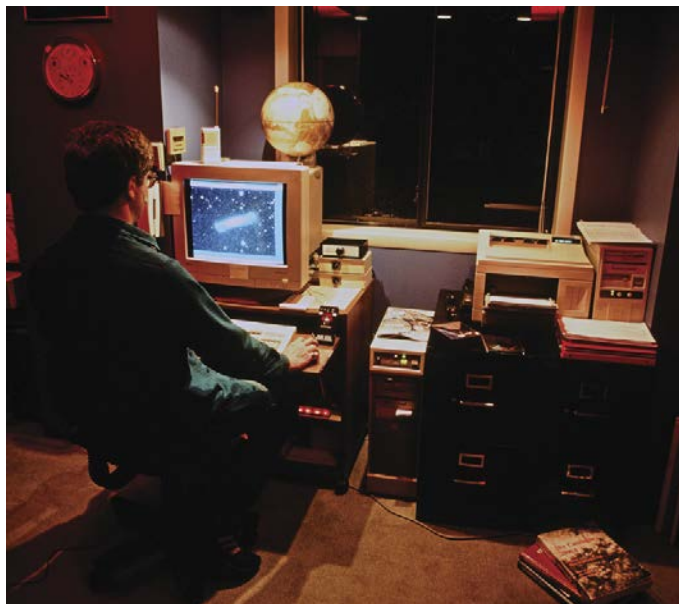
▲ Left: By the mid-1990s, CCD cameras controlled by a desktop computer began to supplant 35-mm film as the medium of choice for cutting-edge astrophotography. Right: By the middle of the first decade of the 21st century, laptop computers were the brains of most CCD-imaging systems, permitting more portable imaging setups.
