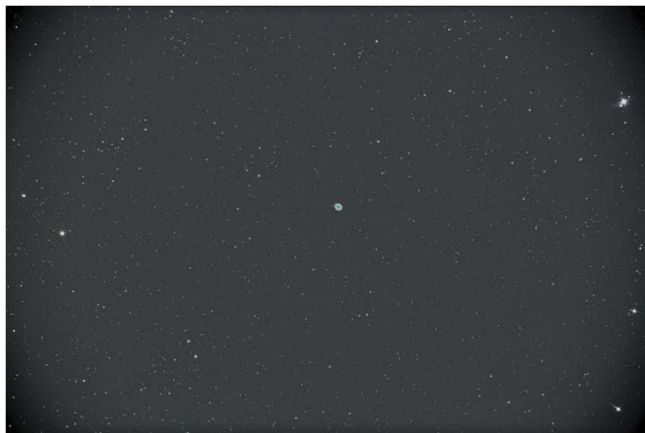
▲ Although there is no dedicated field-flattener for the AT150EDL, the scope still delivers quality star images for many of today's popular astronomy cameras. This stack of three 10-minute exposures of the Ring Nebula, M57, was made with a QHYCCD Minicam 8. It shows the full field of the camera's 11.2-by-6.3-mm CMOS detector that covers a 32'-wide field on this scope. A stack of five 3-minute exposures made with a full-frame Nikon D850 camera ( bottom ) covers a 1.7°-wide field but shows noticeable distortion of the star images at the edges.
