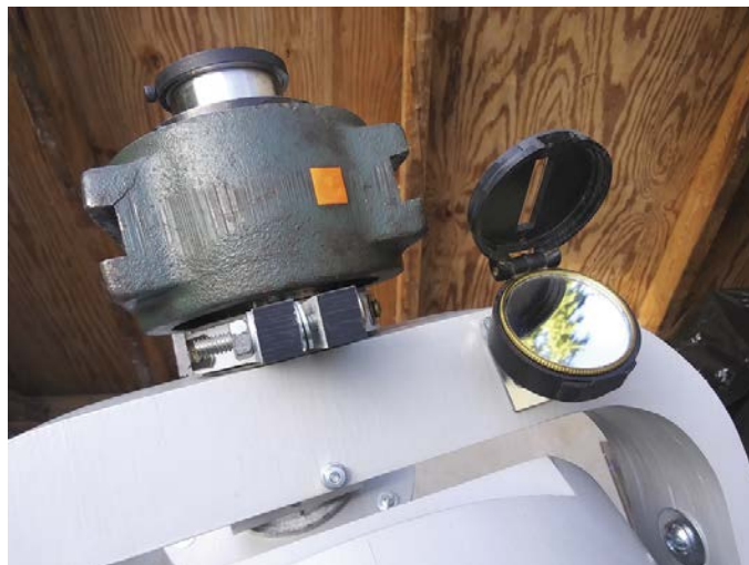
▲ Left: On the left side of the fork, a lag screw interfaces with a modified hose clamp to provide declination axis slow-motion control. Right: An angled mirror on the fork acts as a 1×-power finder in right ascension, allowing Jordan to chase down objects with the slow-motion controls once he located them on the crosshairs.
