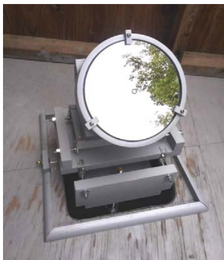
▲ Left: Jordan's 6-inch primary mirror on its three-axis, adjustable mounting. Right: When not in use, the primary mirror is covered with a wooden box.
