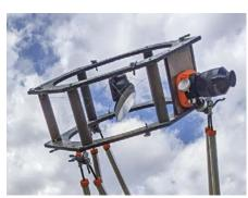
▲ The secondary mirror assembly is held in position with steel wires connected to ukulele tuning pegs.
