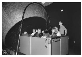
▲ **GROUP EXPERIENCE** The Atwood Sphere allowed for several people to enter a spherical dome in a special cart. The sphere is 17 feet in diameter, and its surface is pierced by 692 holes.
