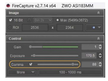
▲ **CONTRAST BOOST** Adjust the *Gamma* slider in your control software (the example shows *FireCapture*) in order to set the midtone contrast before recording your videos.
