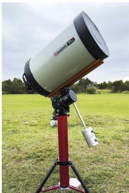
▲ Left: Despite being close to the maximum weight capacity of the 150i, the mount held this Celestron EdgeHD 14-inch OTA, though it required extra counterweights and a sturdier tripod than the one provided by Sky-Watcher. Right: Even without using counterweights, Sky-Watcher's 180-mm Maksutov-Cassegrain was a comfortable match for the 150i when configured with the optional tripod and tripod extension.
