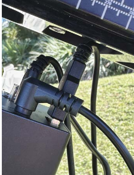
▲ Users should be aware that cables plugged into the control panel can interfere with movement of the declination axis, particularly with scopes fitted with long dovetail mounting bars.
