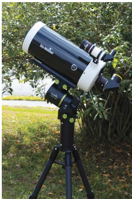
▲ Left: Despite being close to the maximum weight capacity of the 150i, the mount held this Celestron EdgeHD 14-inch OTA, though it required extra counterweights and a sturdier tripod than the one provided by Sky-Watcher. Right: Even without using counterweights, Sky-Watcher's 180-mm Maksutov-Cassegrain was a comfortable match for the 150i when configured with the optional tripod and tripod extension.
