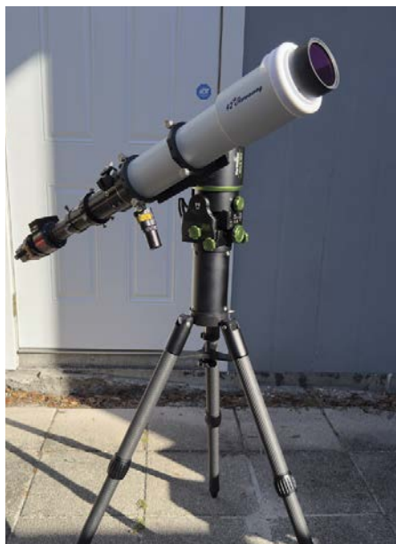
▲ Solar observing and imaging with the 150i was especially easy in alt-azimuth mode. Simply set the mount down with the scope pointed north, make sure your solar filter is in place, then align on the Sun. The author used the 92-mm scope and Player One Apollo-M camera seen at left to image two active regions and filaments seen at right.
