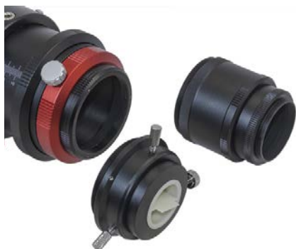
▲ The 2-inch visual back and its 1 1/4-inch insert use brass compression rings to hold eyepieces. A set of camera adapters is also standard. The adapters and the visual back thread onto the focuser's M69-to-M63 step-down ring.
