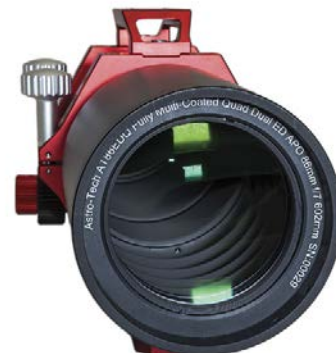
▲ The triplet objective lens and internal flattener are thoroughly multi-coated. The blackened tube interior has five knife-edge baffles, and the focuser includes multiple ribs for additional stray-light suppression.
