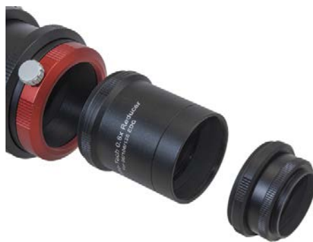
▲ The optional 0.8× focal reducer has a 60-mm diameter lens and threads directly onto the focuser. It needs the step-down rings from the main adapter set to work with M54 or M48 camera nosepieces or T-rings.
