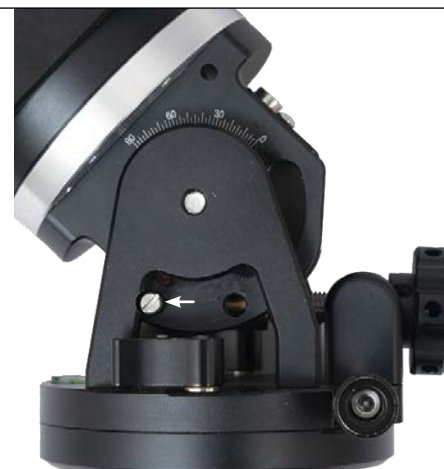
▲ Move the threaded steel pin (arrowed) within the altitude axis from the 45° to the 0° position when switching between alt-azimuth (left) and equatorial modes (right).
