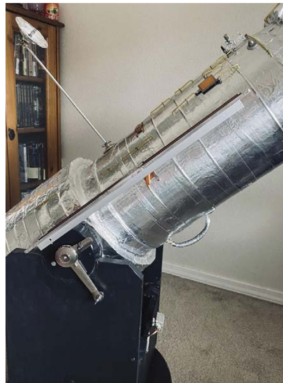
▲ An unobtrusive lid stay eliminates the need for counterweights or springs.
