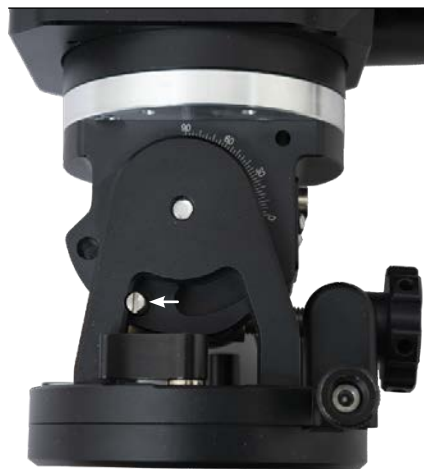
▲ Move the threaded steel pin (arrowed) within the altitude axis from the 45° to the 0° position when switching between alt-azimuth (left) and equatorial modes (right).
