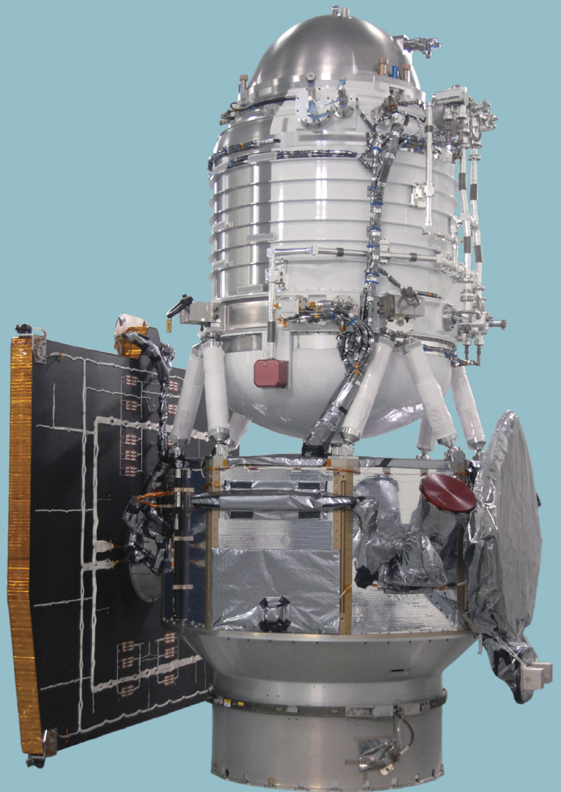
▲ THE SPACECRAFT Seen here in the lab before launch, the WISE space vehicle's white cryostat encloses the instrument and also contains the solid-hydrogen tanks, imaging optics, and detector arrays. The silver dome-shaped cover was ejected shortly after launch.
