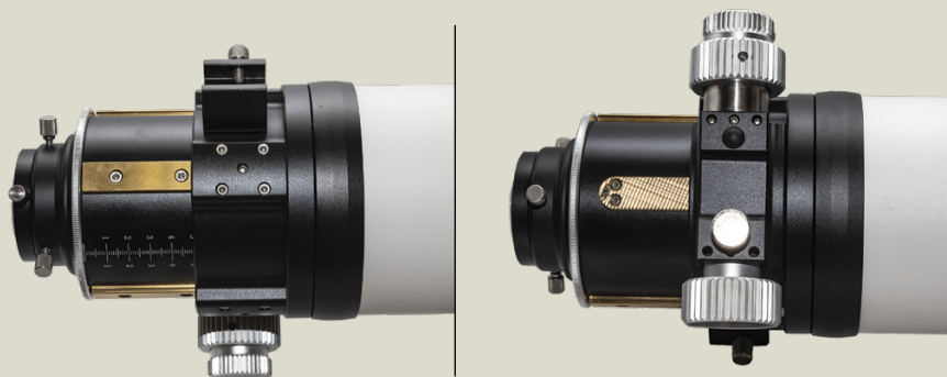
▲ Left: The rack-and-pinion focuser rides along three linear bearings that produce excellent rigidity. Right: a knurled thumbscrew located on the bottom of the gearbox locks the focuser in place.
