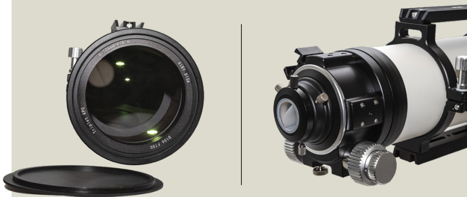
▲ Left: The scope includes two ring baffles to reduce internal reflections. A threaded aluminum lens cap protects the objective when not in use. Right: The heavy duty, 2-inch dual-speed focuser has a bracket for mounting a finderscope or guidescope, though neither are provided. The focuser and its 2-to-1¼-inch adapter use non-marring brass compression rings to secure eyepieces and star diagonals.
