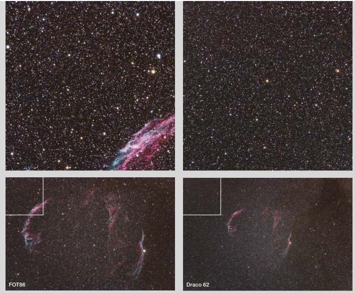
$\blacktriangle$  The FOT86 with its 1× flattener at f/6.5 yielded pinpoint stars to the corners of a full-frame sensor. There was no sign of astigmatism distorting stars into birds! All corners looked the same, with no focal plane tilt.
