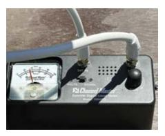
▲ When the IBT is pointed at the Sun, the signal meter registers the influx of radio waves.
