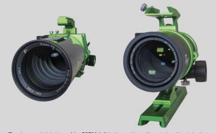
▲ The air-spaced triplet lens of the FOT86 (left) is thoroughly multi-coated and in a tube that is blackened with four knife-edge baffles. The Draco 62's objective (right) is also a triplet, in a blackened and ribbed tube, with a doublet flattener integrated into the rear of the tube.
