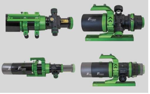
The Draco 62 incorporates an air-spaced triplet objective and a 2-element flattener integrated into its body for a quintuplet Petzval design. Natively, the Draco is f/4.8 with a 300-mm focal length, yielding a 6.8° by 4.5° photographic field. A 0.83× reducer is included with the scope which employs just a single, thick meniscus lens. Using it yields a focal ratio of f/3.9 and a focal length of about 250 mm.
