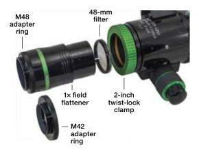
**♦►** Left: The FOT86's 1× flattener accepts 48-mm (2-inch) filters and comes with a choice of M48 and M42 camera-side adapter Rings. Right: The Draco 62 has two camera adapters, with M48 and M54 cameraside threads. The M64 ring is required when shooting at f/4.8, but not when using the reducer, which threads into the focuser. Either adapter ring then threads over it. The reducer and the M64 ring each accept 2-inch filters.
