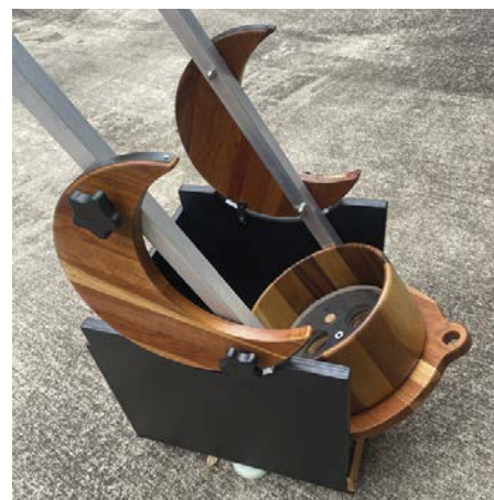
▲ Left: Cindy used a gorgeous hardwood bowl and cutting boards for the mirror enclosure, its base, the altitude bearings, and the secondary ring. Right: The focuser mounts on slotted angle brackets for adjustability.
