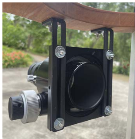
▲ Left: Cindy used a gorgeous hardwood bowl and cutting boards for the mirror enclosure, its base, the altitude bearings, and the secondary ring. Right: The focuser mounts on slotted angle brackets for adjustability.
