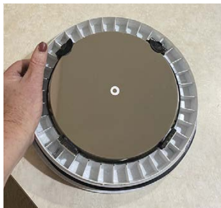
▲ The primary mirror rests securely in its bucket-lid cell.
