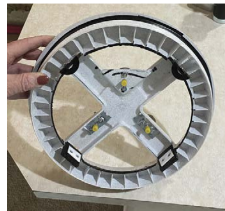
▲ The bucket lid makes an excellent primary mirror cell.
