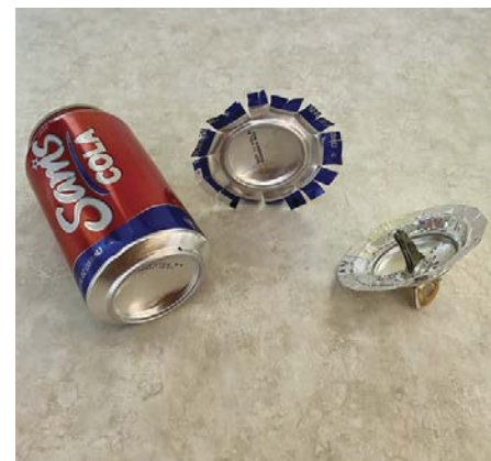
▲ The bottom of a Sam's Cola can covered in foil made a perfect dish antenna.
