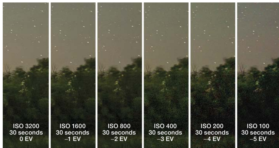
▲ Beginning with a properly exposed shot at far left, each image progressing towards the right was underexposed by -1 to -5 EV by lowering the ISO, then brightened during processing by +1 to +5 stops to compensate. An underexposure of -3 EV proved to be the Z6III's limit when lifting dark shadow content.
