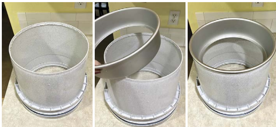
▲ A bottomless cake pan fits within the bucket perfectly and provides a firm seat for the upper tube assembly.
