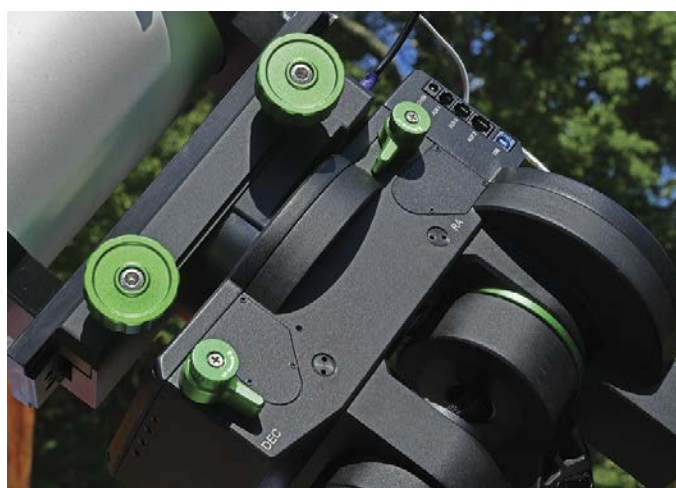
▲ Levers on the side of the declination assembly operate clutches on both axes that completely disengage the drive worms from their respective worm wheels, thus making easy work of balancing the telescope load. Both clutch levers are fitted with knobs that lock the levers in place and help prevent the clutches from being accidentally disengaged.
