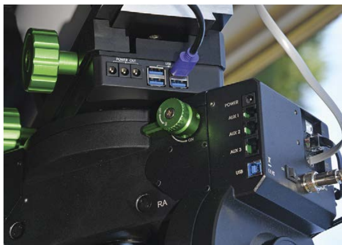
▲ Cable connections on the side of the declination assembly have through-the-mount wiring to corresponding ports on the telescope saddle. Included are hub ports for four powered USB 3.0 connections, three power outlets (fed from the single power jack on the declination assembly), and modular jacks for RJ10, RJ12, and RJ45 (4-, 6-, and 8-pin, respectively) connectors that are on the side of the saddle and not visible in this view.
