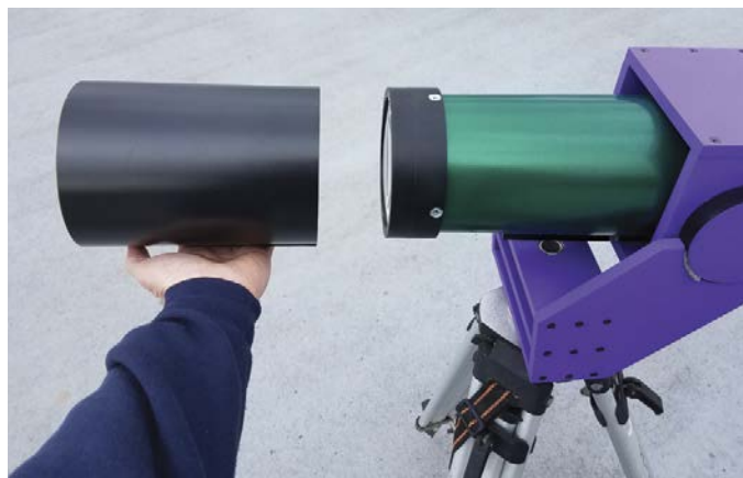
▲ Make the dew shield at least the length of the tube diameter and wider than the diameter of your lens.
