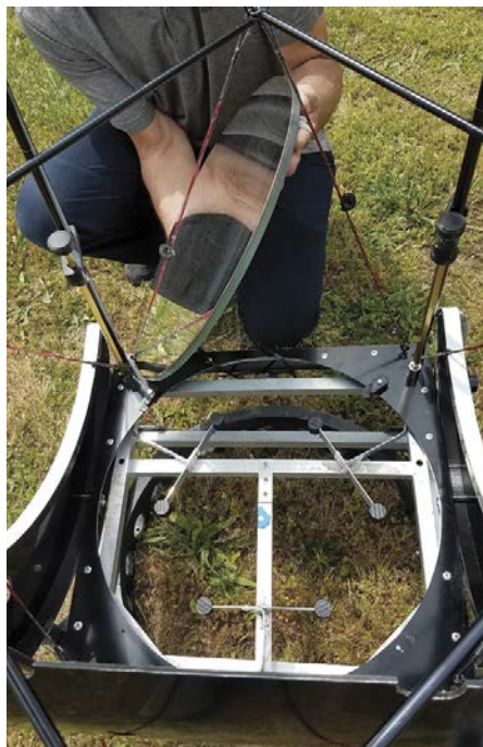
▲ The 6-point mirror cell uses twisting flexure instead of loose parts. The mirror is ½-inch-thick soda-lime glass slumped to f/2.8, provided by DOTI Optics ( doti-optics.com ).
