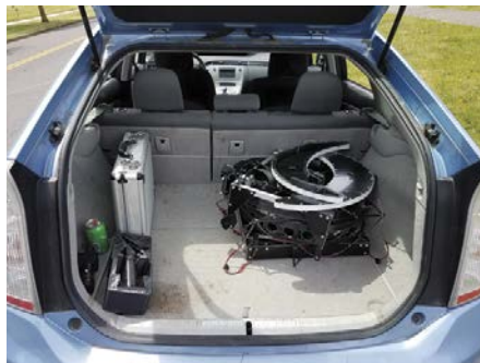
▲ An ultra-lightweight mirror and a tensegrity structure make this scope more portable than many with half the aperture.
