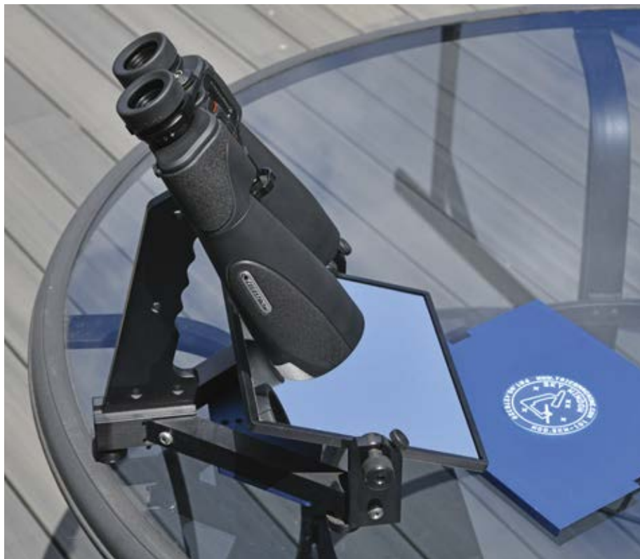
▲ As detailed in the accompanying text, the author used the Sky Window binocular mount when observing celestial objects at high altitudes. This device provides comfortable viewing at the expense of views that are upside down and mirror-reversed.
