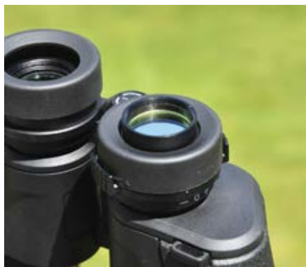
▲ The SkyMaster Pro binoculars have eyepieces threaded to accept standard 1¼-inch astronomical filters, such as the dual-band nebula filter seen here with the eyecup retracted (left) and fully extended (right). The extended position may keep your eyes too far back to allow seeing the full field of view, especially if you need to wear eyeglasses when observing.
