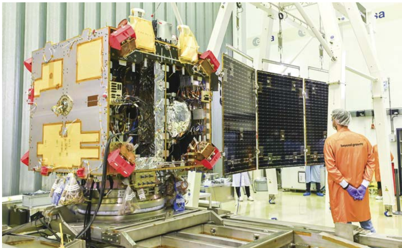
▲ HERA STRETCHES A WING Team members inspect the Hera spacecraft with one of its two solar-panel wings attached. The panels are supported here by a frame because they're designed to operate in zero gravity.
