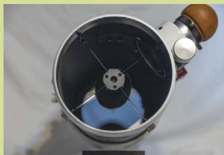
▲ The secondary-mirror assembly uses three hex-head bolts for adjusting its tilt, and the central post is affixed using a Philips-head screw, which lets you shift the position of the secondary back and forth — both important adjustments for any Newtonian. In addition, a white ring marks the center of the primary mirror to aid collimation.
