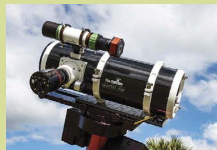
▲ For imaging use, the Quattro 150P easily supports an average-size modern CMOS camera or crop-sensor DSLR camera. The shoe for the 6 × 30 finderscope also accepts guidescopes, such as the Evoguide 50DX model seen here (and reviewed in our June 2022 issue, p. 70).
