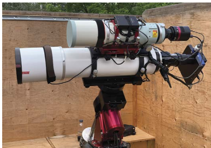
▲ WIRED FOR ACTION In addition to his robotic telescope mount, all the author's equipment is connected to the Eagle 4 Pro imaging PC and accessed wirelessly. The control box for the focuser is located atop the smaller scope.
