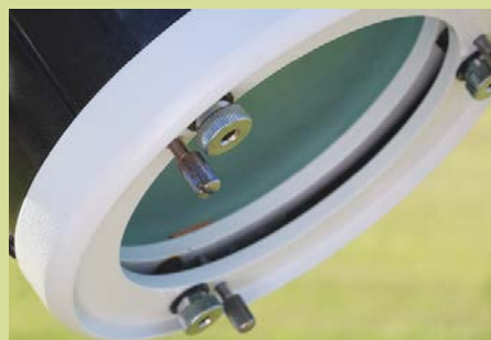
▲ Collimation of the primary mirror is performed with the three large, spring-loaded knobs on the rear of the cell and secured with the three taller knurled knobs. The taller knobs quickly began to rust in the author's humid Florida environment.
