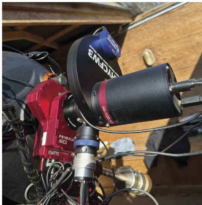
▲ BUSY IMAGING TRAIN Several devices are necessary to permit imagers to have the most options when composing astrophotos. Seen from left to right are PrimaLuceLab's ESATTO low-profile focuser and ARCO camera rotator, an off-axis guider with a QHYCCD guide camera, a 7-position filter wheel, and the main QHY600M imaging camera.
