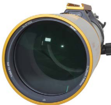
▲ Left: The scope's 120-mm (4.7-inch) triplet objective is anti-reflection coated. Its tube interior is fully blackened with a ribbed section in the upper portion and three field stops all working together to produce good suppression of stray light. Right: The 9-inch-long dew cap retracts onto the tube but extends beyond the lens by 4 inches. It has a locking knob to secure it firmly in position.
