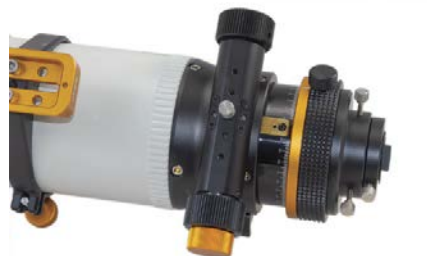
▲ The bottom Vixen-standard dovetail bar is drilled with numerous holes for adjusting the ring spacing if desired. The rack-and-pinion focuser has a lock knob, tension screws, and M4-threaded holes for attaching electronic focusers.
