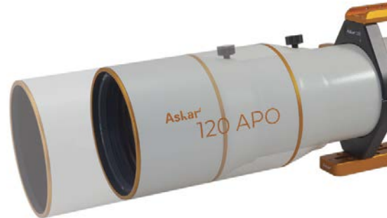
▲ Left: The scope's 120-mm (4.7-inch) triplet objective is anti-reflection coated. Its tube interior is fully blackened with a ribbed section in the upper portion and three field stops all working together to produce good suppression of stray light. Right: The 9-inch-long dew cap retracts onto the tube but extends beyond the lens by 4 inches. It has a locking knob to secure it firmly in position.
