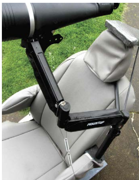
▲ Left: Bracing rods between the chair and the monitor arm provide stability and vibration damping. Springs counter the extra lift of the monitor stand's internal springs. Lauren moved the nameplate from the top section to the lower section to cover the spliced length of metal pipearm ( middle ) added to extend the monitor arm's reach. Right: Lauren added a gyroscope in order to dampen rotational vibrations.
