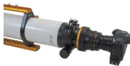
▲ Top: Removing the rear section of the main tube allows binocular viewers (a Baader unit is shown) to reach focus without needing a Barlow lens. Bottom: The extension tube is required for either of the photographic flatteners to reach focus.
