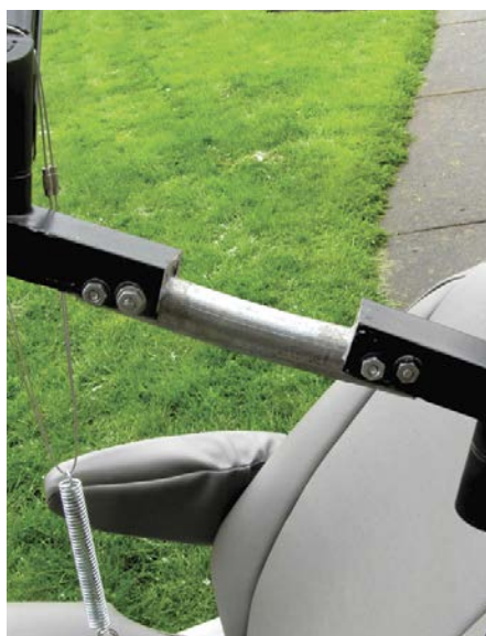
▲ Left: Bracing rods between the chair and the monitor arm provide stability and vibration damping. Springs counter the extra lift of the monitor stand's internal springs. Lauren moved the nameplate from the top section to the lower section to cover the spliced length of metal pipearm ( middle ) added to extend the monitor arm's reach. Right: Lauren added a gyroscope in order to dampen rotational vibrations.
