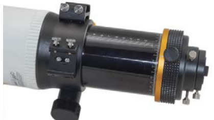
▲ The slotted top plate accepts accessories with Synta-standard dovetail feet. The back of the tube has two additional finder bases. The 3.3-inch focuser offers 100 mm of travel and has graduated scales for focus position and rotation angle.
