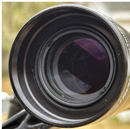
▲ The StarSense Autoguider has a 28-mm effective-aperture objective lens with a focal length of 120 millimeters. This produces a plate scale of 4.98 arcseconds per pixel.
