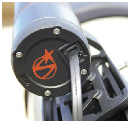
▲ The rear of the StarSense has two ports: a USB-C receptacle for interfacing with a PC (left) and an RJ-11 port (right) for the auxiliary cable used to connect to your Celestron mount. The device also includes built-in Wi-Fi.
