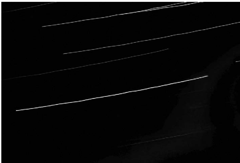
▲ This 25-minute trailed-exposure test is described in the text. Recorded with the author's 90-mm, 1,250-mm-focal-length Maksutov-Cassegrain, it shows nearly straight star trails, confirming the polar drive's low periodic error.
