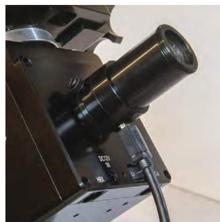
▲ Left: The north-facing side of the mount includes the jack for the Go2Nova hand controller, an ST-4 autoguiding connection, and the 12-volt DC power input as well as the on-off switch. At top is the bubble level required for leveling the head when setting up in alt-azimuth mode. The level also serves as a mounting stud for the iPolar camera. At bottom is the \frac{3}{8} \times 16 threaded socket that accepts an optional 200-mm long counterweight bar. Right: This image shows the iPolar polar-alignment camera installed and secured by its two thumbscrews. A Mini-USB cable connects the device to a PC computer running the iPolar software.
