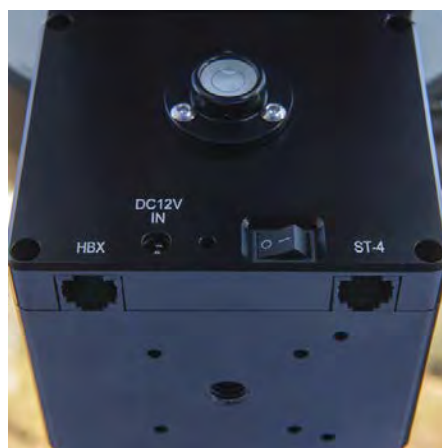
▲ Left: The north-facing side of the mount includes the jack for the Go2Nova hand controller, an ST-4 autoguiding connection, and the 12-volt DC power input as well as the on-off switch. At top is the bubble level required for leveling the head when setting up in alt-azimuth mode. The level also serves as a mounting stud for the iPolar camera. At bottom is the \frac{3}{8} \times 16 threaded socket that accepts an optional 200-mm long counterweight bar. Right: This image shows the iPolar polar-alignment camera installed and secured by its two thumbscrews. A Mini-USB cable connects the device to a PC computer running the iPolar software.
