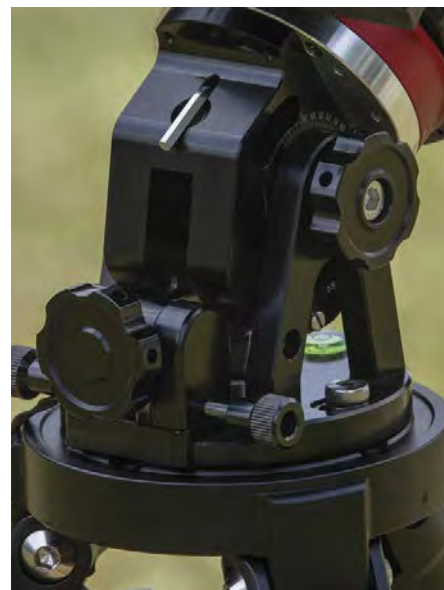
▲ This rear view of the HAE29EC shows the azimuth and altitude adjustment knobs and the stowed hex wrench that fits most of the screws on the mount. The hole on the side of the altitude plate is for storage of the azimuth-locking screws when not attached to the tripod.
