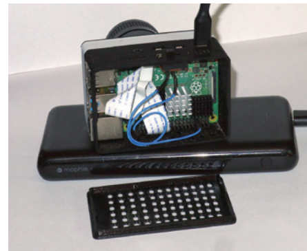
▲ The Raspberry Pi computer and the camera fit comfortably in a 3D-printed box measuring 2.5" × 3.5" × 2".
