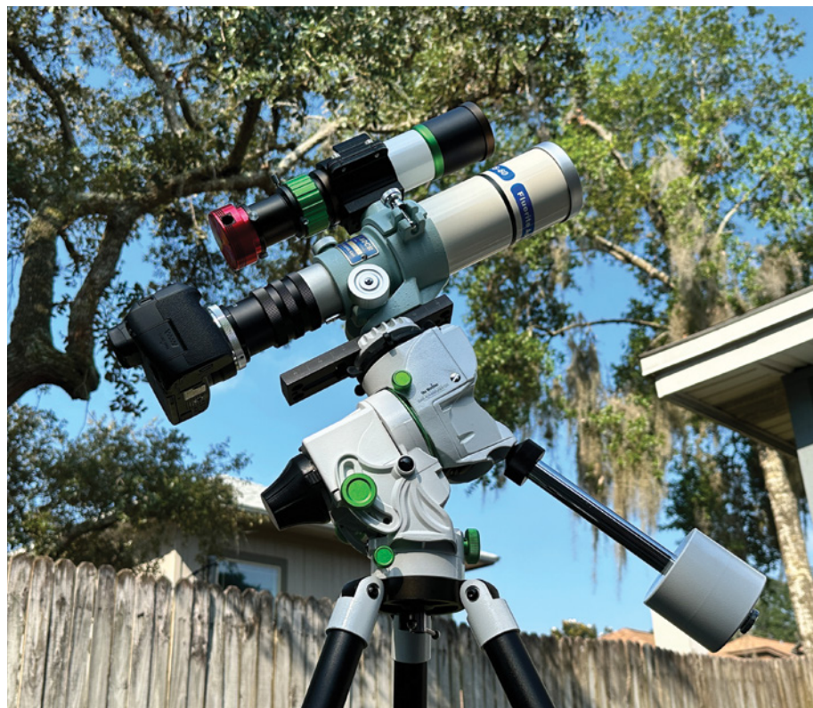
▲ The Star Adventurer GTi easily accommodates the author's Takahashi FS-60 refractor and piggy-backed EvoGuide 50ED guidescope (reviewed in our June 2022 issue, page 70). The combination is well under the 5-kg weight capacity of the mount.
