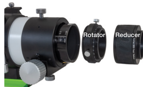
▲ The optional reducer/corrector comes in two parts: the camera rotator, which screws onto the 62-mm threads of the focuser, and the 0.9× field flattener itself, which attaches to the 56-mm threads of the rotator and provides a standard 48-mm thread on the camera side for T-ring adapters and camera nosepieces.
