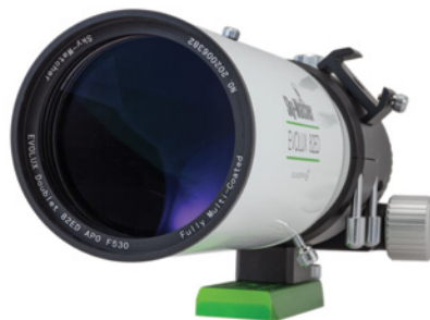
▲ The 82mm ED doublet objective is multi-coated and the interior of the tube blackened, though without any ring baffles or interior ridges to help suppress stray light.
