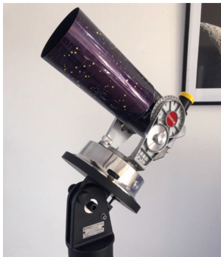
▲ The Questar telescope mounts to a solid aluminum disk. Polar alignment is adjustable with a fine-tuning bolt.
