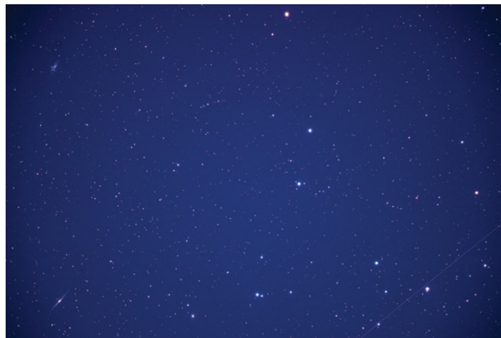
◀ A single exposure with a full-frame sensor (the Canon EOS Ra) taken in twilight shows the level of vignetting when using the reducer/corrector, with the combination offering a fully illuminated field of 36 mm.
