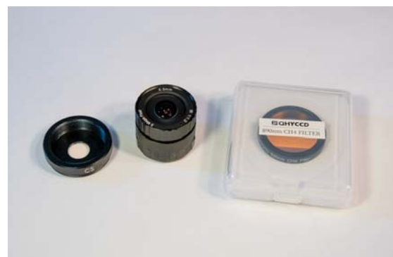
▲ The expansion kit for the QHY5III462C includes a replacement window with UV/IR blocking, a 2.5-mm f/1.5 all-sky lens, and a 1¼-inch 890-nm CH 4 (methane) filter, which is useful for recording deeper features within Jupiter's atmosphere.
