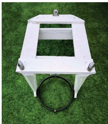
▲ The three trolley wheels are angled to allow circular motion but resist sideways motion.
