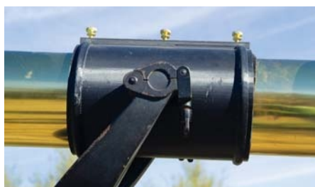
▲ The 3D-printed mounting cradle fits in beautifully with the rest of the scope.
