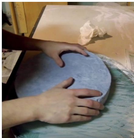
▲ Zane's second completed scope is a 16-inch f/5 (seen at left), which required that he refigure the primary mirror (right).
