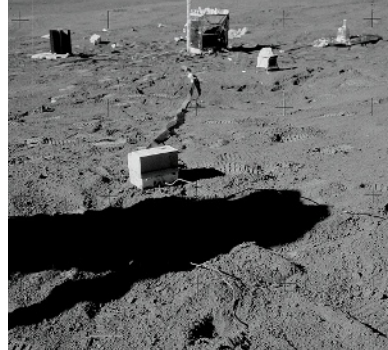
▲ This image of Apollo 15’s ALSEP setup shows the HFE power box in the foreground. Cords to the detectors snake off to the lower right. The foreground shadow is that of astronaut David Scott.
