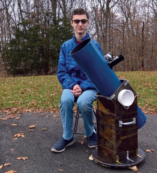
▲ Zane Landers with his first home-built, hand-polished 6-inch f/5 telescope.
