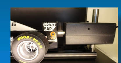
Force sensor: measuring air resistance.
