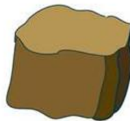
Massive (low permeability)
