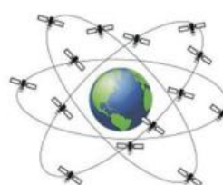
Galileo 3 Orbital planes 27 Satellite + 3 Spares 56° Inclination Angle Altitude 23,616 km
