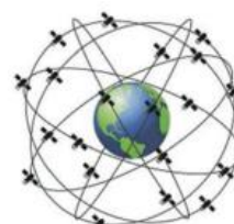
GPS 6 Orbital planes 24 Satellite + Spare 55° Inclination Angle Altitude 20,200 km
