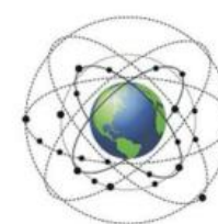
BeiDou 6 Orbital planes 35 Satellite + 3 GEO + 27 MEO + 3 IGSO 55° Inclination Angle Altitude 38,300 km, 21,500 km
